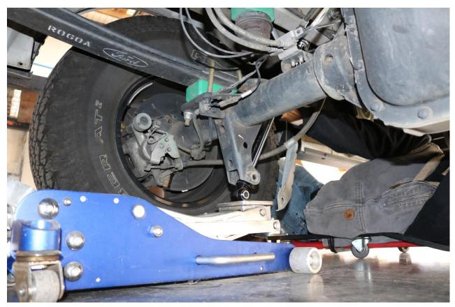
10) Install the OEM lower shock bolt from the outside so the nut is towards the inside of the vehicle.
