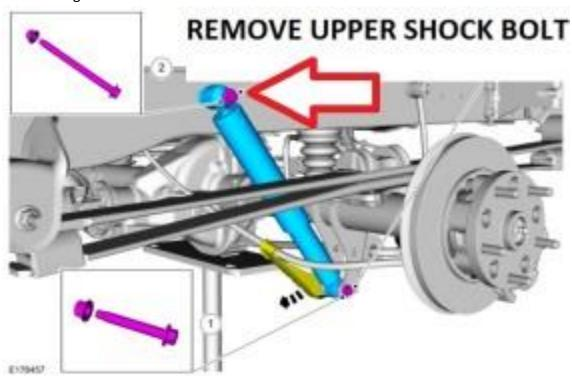
5) Note the Falcon shocks are left and right specific, refer to the part number etched on the shock body to ensure they are installed on the correct side.
