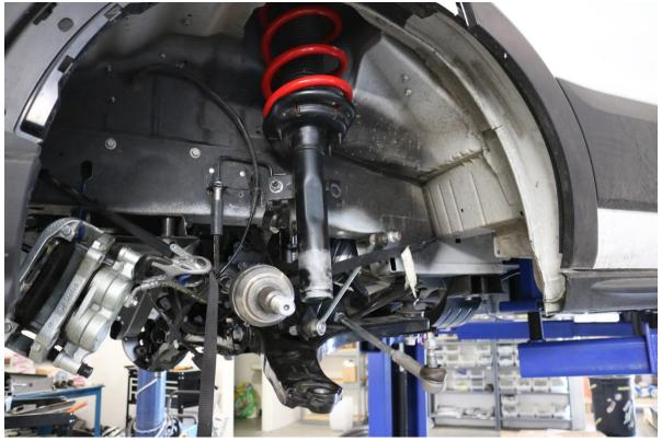
16) Remove the three upper strut nuts securing the strut to the chassis. Use a 15mm socket / wrench for removal (13mm for 2013-2017). On the driver (left hand) side of the vehicle, the nuts are accessible via the driver foot well.
