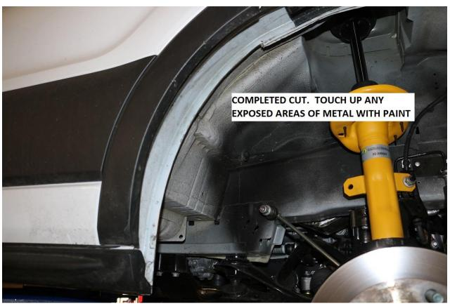
43) Towards the front of the wheel opening, locate the inner M6 bolt securing the front bumper fascia to the vehicle. There is a small flange that needs the corner cut off. Note, the outer fender trim piece is removed in this photo for clarity.
