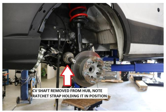
15) With the CV free from the hub, support the steering knuckle with a transmission or floor jack and remove the 18mm lower strut bolt. Remove the steering knuckle from the strut and set it aside.
